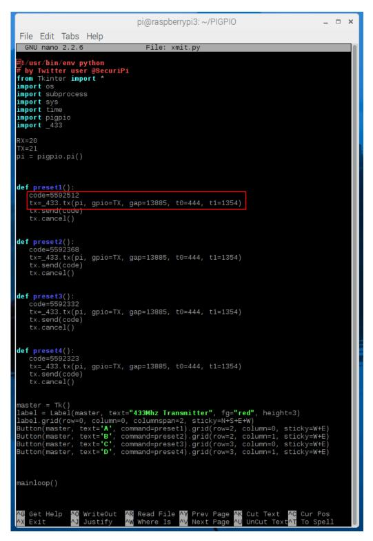
This is the python script xmit.py running on the Pi's desktop. You can use it to send button codes to the receiver module that came with the 433Mhz keyfob.
