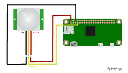
The wires you use may vary in colour from those shown above. Connect VCC to 5V, OUT to GPIO4 and GND to GND. Pin labels are screen printed on the PIR's circuit board – lift the plastic dome off if you don't see them. The two trimmers on the top of the PIR allow you to change the sensitivity & dwell time of the PIR, leave them set at defaults for now.
