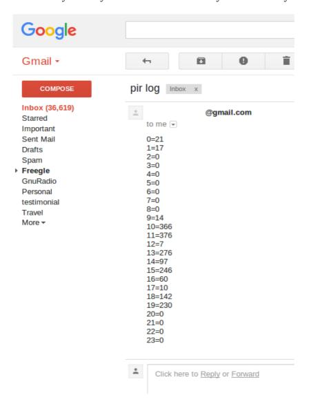
As you can see from the picture above, our demo person didn't trigger the PIR between sometime after 1am until sometime after 9am. Also, they didn't trigger the sensor between 8pm and midnight.
