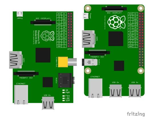
The older Pi model B is on the left in the above photo. It has a total of 26 GPIO pins, arranged 2x13.
