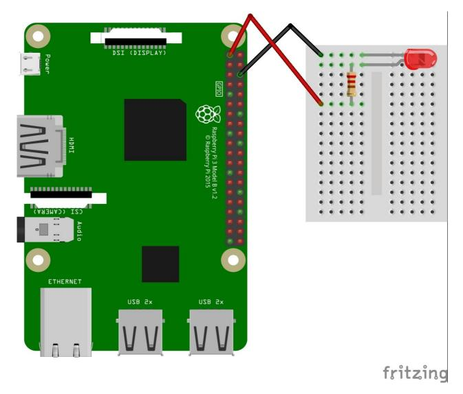
When you're happy the red LED is working correctly, you can also test the yellow & green LEDs.
