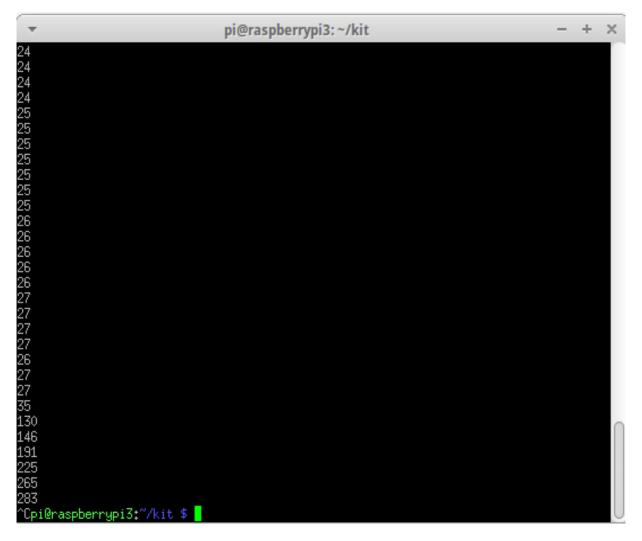
We can use this LDR experiment as the basis for a drawer or cupboard alarm, and have the Raspberry Pi email us when the light level changes from darkness (200+) to daylight (less than 50).
