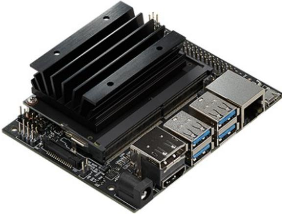
The board has a 40 way GPIO edge connector that's compatible with the Raspberry Pi. Here's how you set it up and use it:
