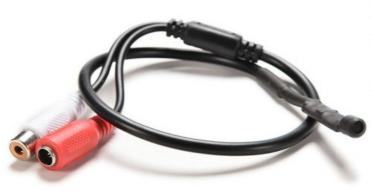
The CCTV mic is powered by a 12 volt DC supply. It contains a microphone and an amplifier. The 12V supply attaches to the red 2.1mm plug. The white phono socket attaches to a USB soundcard with a Line Level input.
