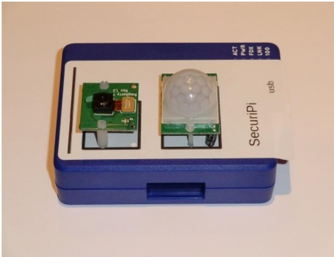
It doesn't matter if the Pi camera is physically mounted upside-down, as the image can be flipped horizontal or vertical with a command line switch of `-hf` or `-vf`. The only important thing is that the CSI camera cable reaches without too much tension on it. The positioning shown in the photo worked fine for us.
