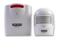
The receiver unit has a sounder and several red LEDs that buzz & flash to alert you of alarm outside. We remove one of the red LEDs and feed the signal into the H11L1 chip.
