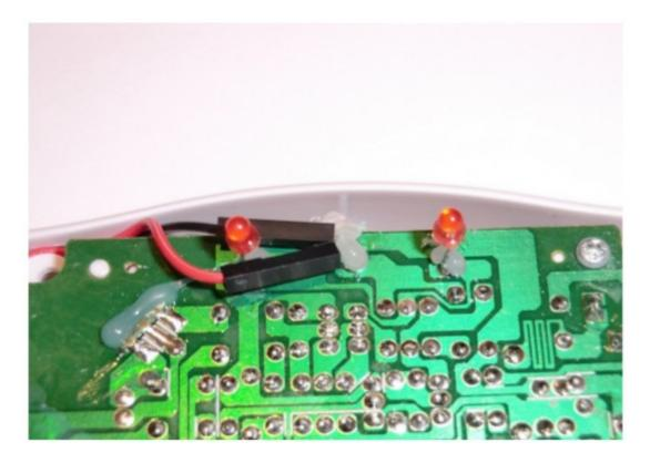
We've removed the cover and cut the head off the centre red LED and attached to IDC cables (included with kit).
